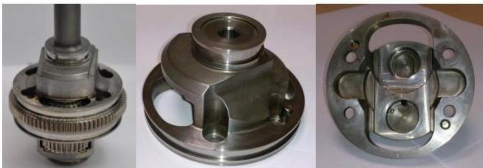
Figure 1 Assembled carrier shaft of the CSD (left) and parts considered for additive manufacturing (centre and right). Source: CU
